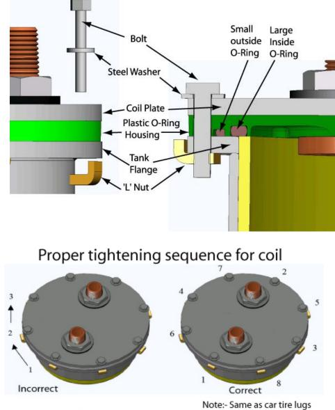
Caution: Does not require excessive force to seal properly.
