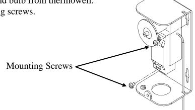
7. Replace thermostat using reverse procedure. (Note: Be sure to place capillary tube into slot in base prior to installing cover.)
