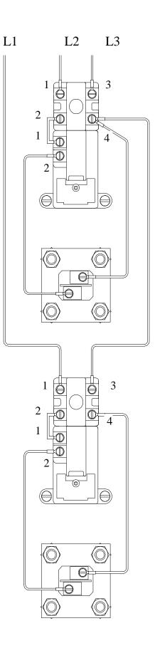
3 Ø Open Delta Wiring for Simultaneous Operation
