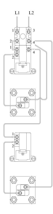
Interlocked for Non-Simultaneous Operation
