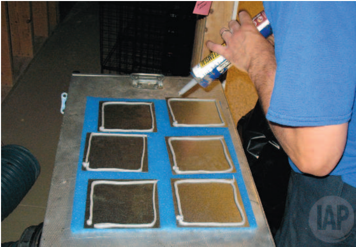
Silicone caulk tightly seals all cover plates.
