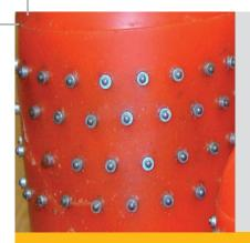
One of the major challenges plant operators are facing is the continuous build-up of coke deposits along the inner wall of furnace tubes. Without service and maintenance, these coke layers grow in thickness, restricting flow of process fluids and increase pressure across the furnace.
