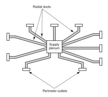
Figure 1. Radial duct system
