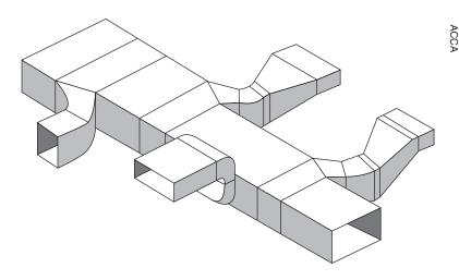
Figure 6. Reducing trunk duct system
