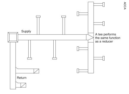
Figure 7. Primary-secondary trunk system
