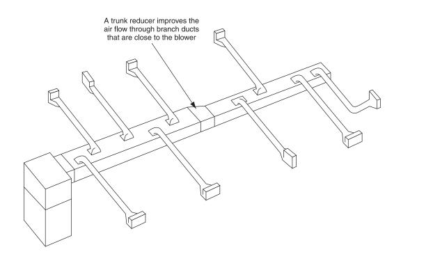
Figure 4. Reducing plenum duct system
