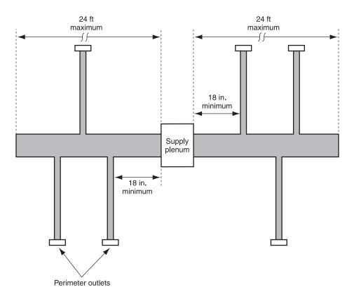
Figure 3. Extended plenum duct system (double plenum)
