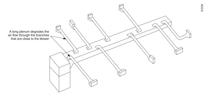
Figure 2. Extended plenum duct system (single plenum)
